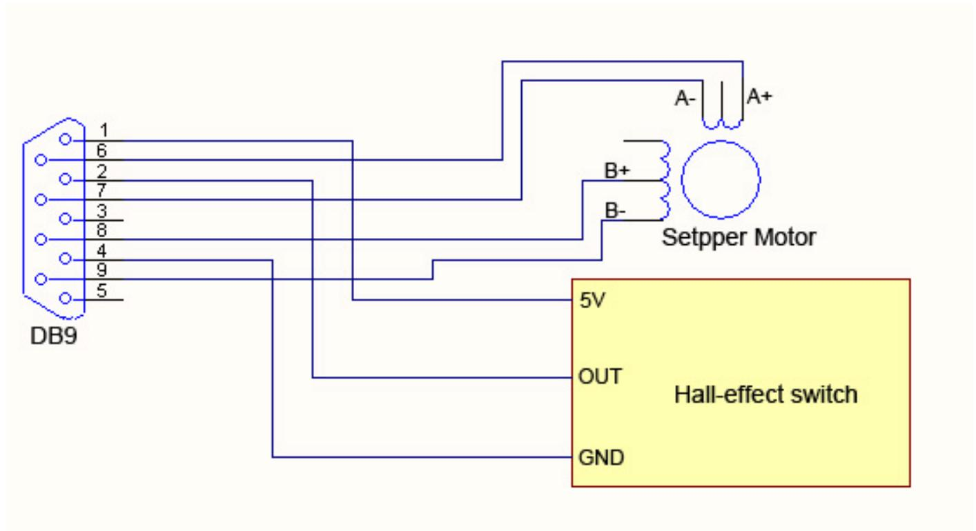
Input voltage of hall effect switch: 5V
