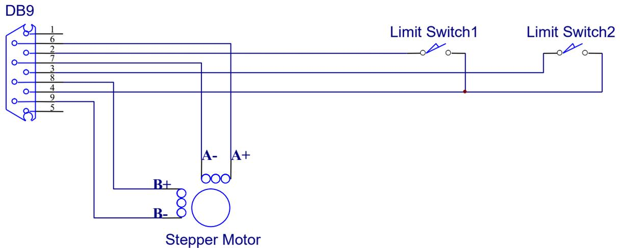
Limit Switch 1 is at the end of the stepper motor. It's the home (zero) position.
